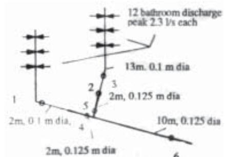
Figure 1: Part of Drainage System
